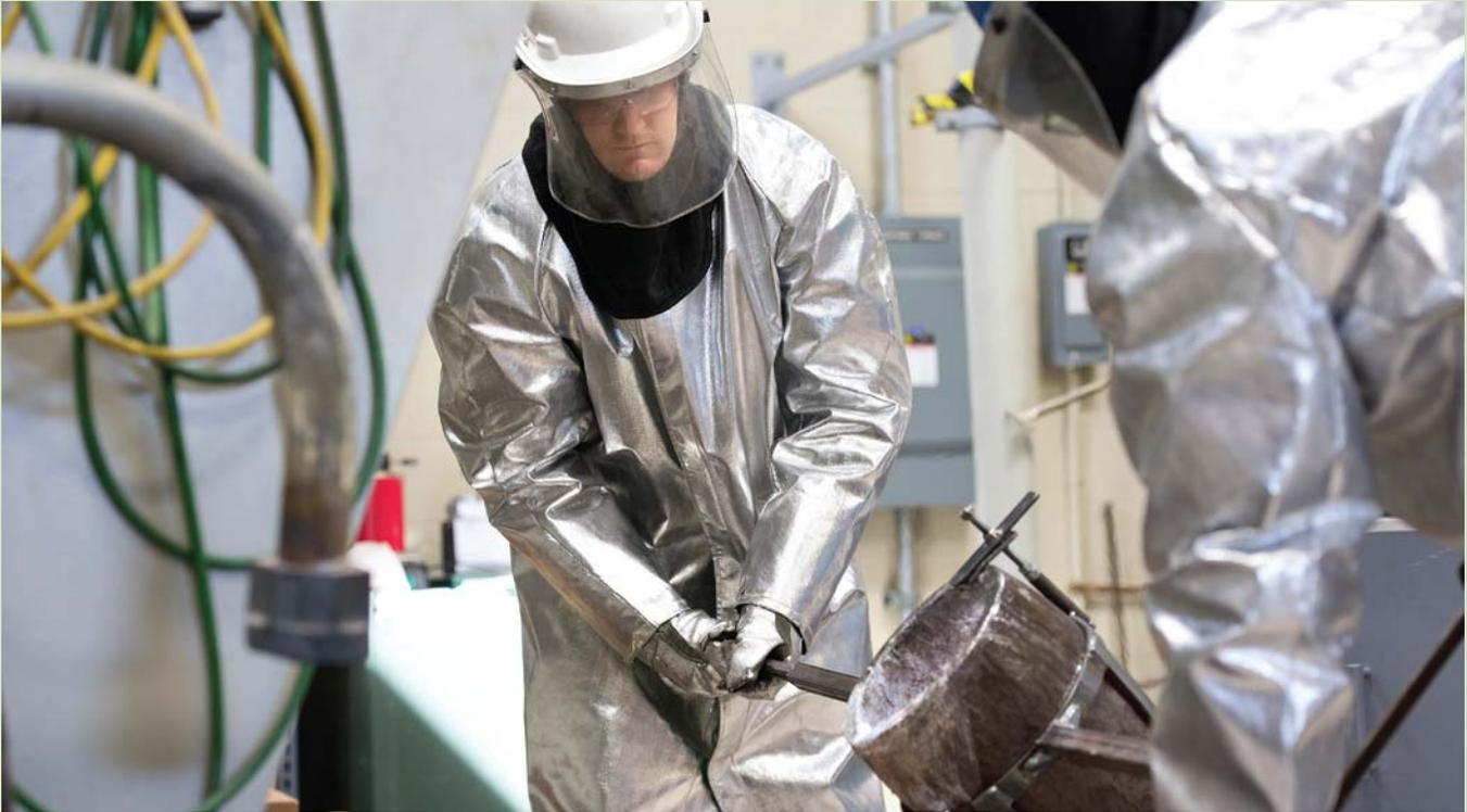
*Drew Snelling uses a common aluminum alloy melted to a temperature of 1,400 degrees to create the final mold, a web-like brick structure that is hoped could be useful for manufacturing (below).*
