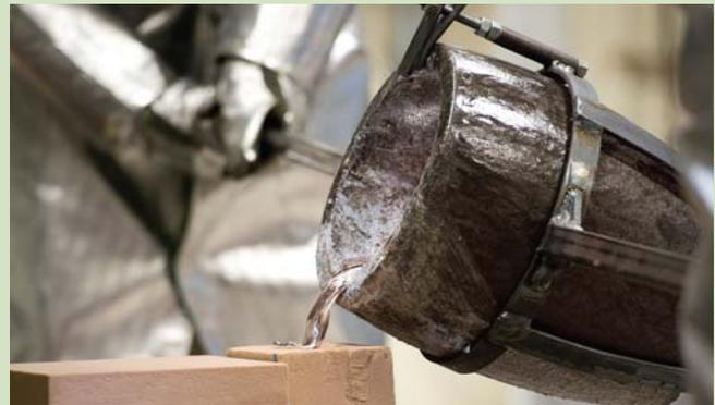
Doctoral student Drew Snelling and Associate Professor Christopher Williams, both of mechanical engineering, use a 3-D printed sand mold to cast metal to create an aluminum-alloy brick that may be used for vehicle armor.
